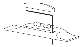
2. Remove only enough material from the width of the saddle to provide a sliding fit in the slot. To test the fit, the saddle should slide easily in the slot, but should not fall out when overturned. To maintain your current action, the new saddle must be .048" shorter in height than your current saddle.
