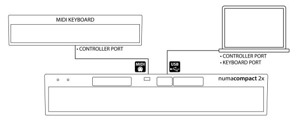
All real time Panel controls (Organ Drawbars and Synth Sliders, SOUNDS, FX selection and related Amounts and settings etc) are sent and received, as listed in the MIDI IMPLEMENTATION CHART. The last four potenziometers are only for local settings (VOLUME, MASTERING, BASS & TREBLE) as they should not be sent or received via MIDI.
