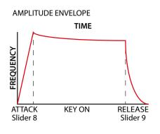
The last two sliders are controlling the ATTACK and DECAY of the AMPLIFIER and they do not change the FILTER parameters, that have separate A/D/R controls; they are able to create Slow attacks and Long release effects, without any change on the FILTER settings.
