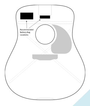
Clean the area where you will mount the bag with an alcohol wipe or cotton swab moistened with rubbing alcohol. Let dry.
