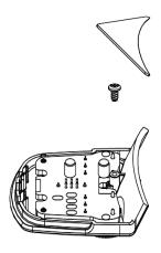
On the back end of the module, remove the 1.5mm hex screw and place it aside as you will need this screw to attach the classical cover.
