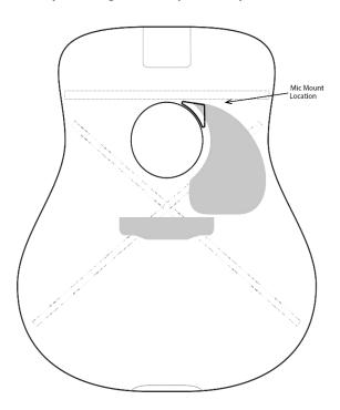
Test the area where you will mount the mic module. Remove any lacquer and/or buffing compound from this area using fine grit sandpaper. Clean this surface with an alcohol wipe or a cotton swab moistened with rubbing alcohol and let dry.
