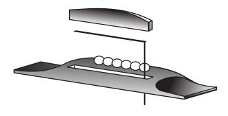
Remove only enough material from the width of the saddle to provide a sliding fit in the slot. To test for proper fit before stringing the instrument, turn the instrument upside down. The saddle should remain in the slot. You should be able to remove it easily with your fingers. If you need tools to remove it, it's too tight!
