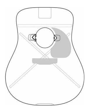
Test the area where you will mount the Volume & Tone control module. Remove any lacquer and/or buffing compound from this area using fine grit sandpaper. Clean this surface with an alcohol wipe or a cotton swab moistened with rubbing alcohol. Let dry.
