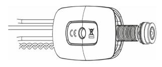
Fasten the Preamp/Jack in the Endpin Hole
