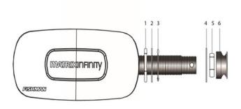
Thread the large nut, dress washer and star washer down the jack towards the preamp body to allow the proper amount of the jack to go through the end block.
