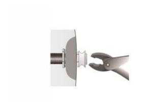
**Note:** With the strap button in place, the end of the jack should protrude slightly, so that when a plug is inserted, it will snap securely in place.
