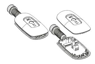
Bring the pickup wire out through the soundhole and fasten it to the terminal block on the preamp module.
