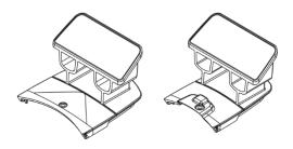
To convert the steel string mounts to classical mounts, remove the adhesive on the cover to expose the small Philips head screw. Remove and place the screw aside as you will need it to attach the classical cover.
